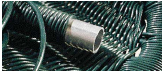
Extruded virgin vinyl wrap over extruded and cold drawn aluminum tubing
